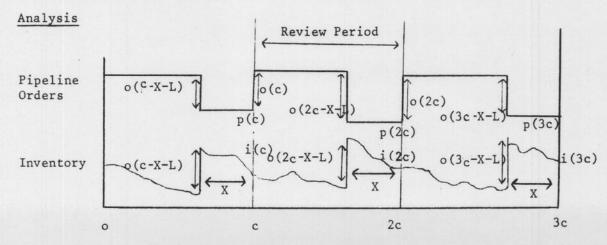
The characteristic of a cyclic review system with fixed lead time is that for an individual company it operates as shown in the figure. Since in the further analysis we wish to use Laplace Transforms we assume for simplicity - without serious loss of generality - that prior to t=0 the system is in equilibrium and that all the values concerned are measured relative to this equilibrium state.
