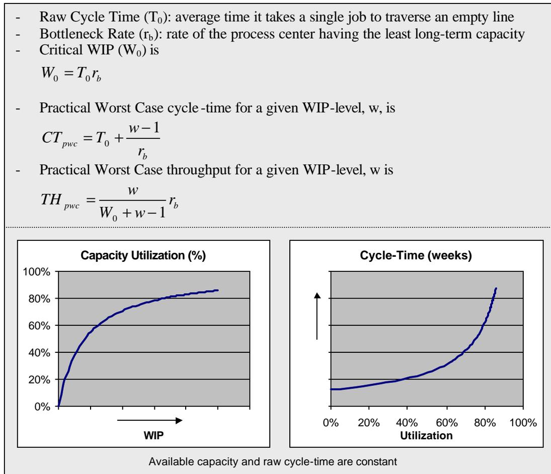
**Figure 4: Key "Factory Physics" for cycle-time and WIP levels (Hopp and Spearman 2000)**
