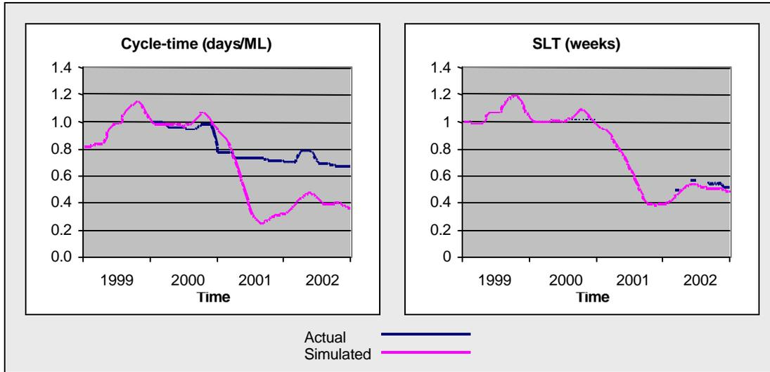
**Figure 12: Simulated and historical behaviour of cycle-time and stacked lead-time**
