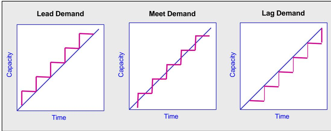
**Figure 14: Different strategies for determining capacity adjustment delays**
