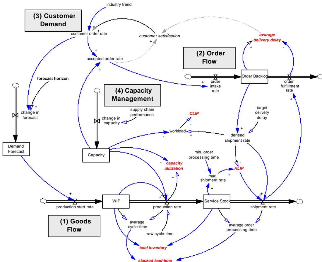
Figure 3: Simplified stocks-and-flow diagram of supply chain model structure
