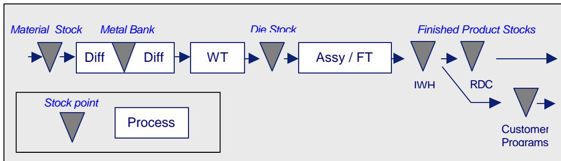
**Figure 5: Semiconductor manufacturing supply chain structure**
