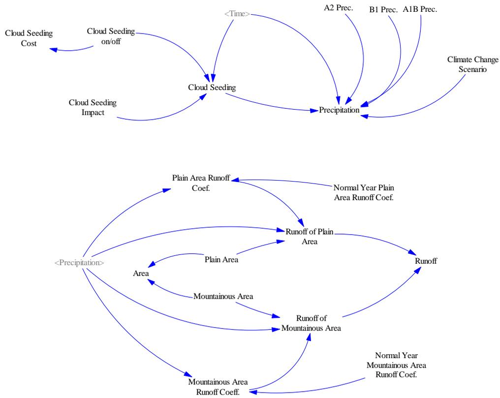
Fig. 4 The sub-models of rainfall and runoff
