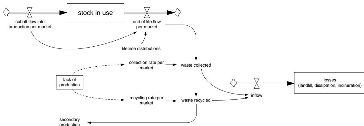
Figure 14 A simplified illustration of the recycling module. Note that the stock in use is only based on lifetime delays of different cobalt end uses. Hence, these stocks are used for material flow simulation without feedbacks from the stocks.
