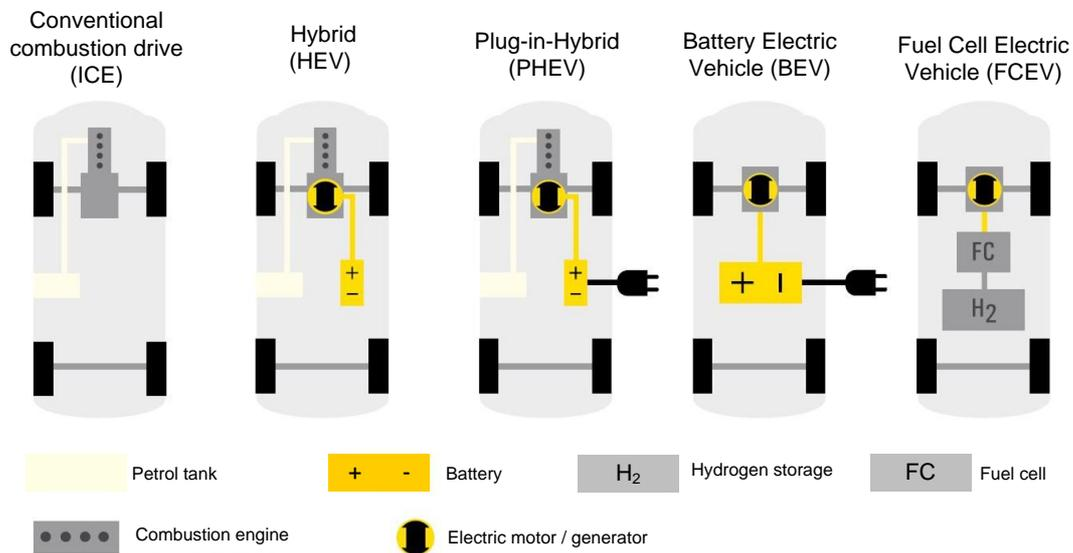
Figure 3 Considered technologies of the Global Mobility Model (GloMo) (Spath et al. 2011)
