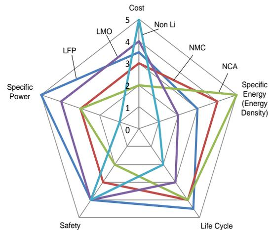
Figure 5 Properties and advantages of different cathode materials (Fraunhofer ISI; based on expert interviews and literature data Tübke 2011, Lamp 2013, Möller 2013, Pillot 2013)
