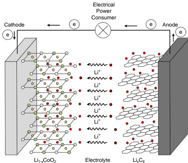
Figure 4 Basic principle of an ordinary Lithium-Ion-Battery with a cobalt oxide cathode material
