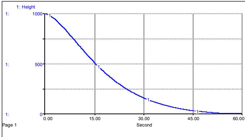
**Figure 14.** Landing behavior generated by the MSD heuristic in the presence of an error in the *Mass* estimate
