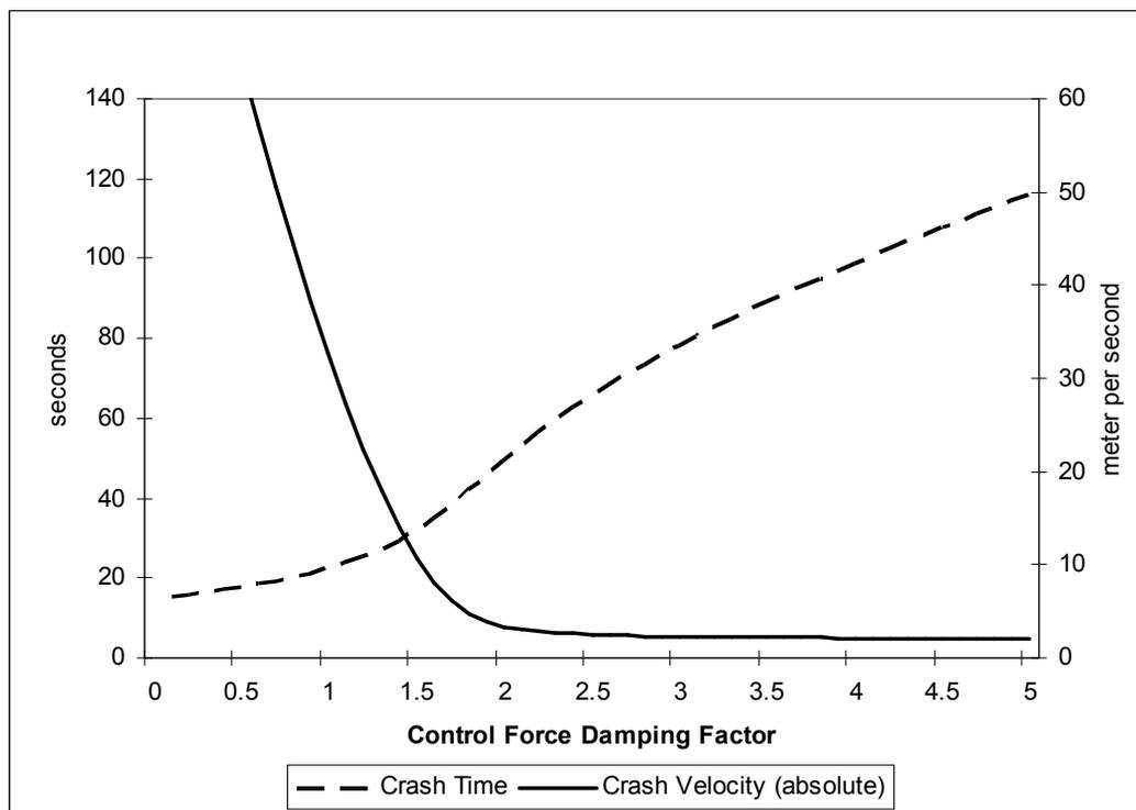
**Figure 5.** *Crash Time* (the time of touchdown) and the absolute value of *Crash Velocity* (the velocity at the time of touchdown) variation with different *Control Force Damping Factor* values
