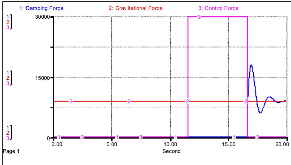
**Figure 13.** Absolute values of the forces acting on the vehicle during landing
