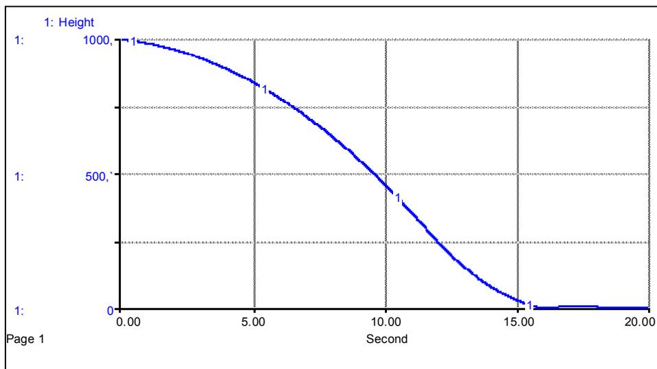
**Figure 15.** Landing behavior generated by the bang-bang heuristic in the presence of an error in the *Mass* estimate
