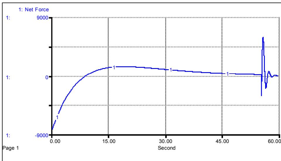
**Figure 8:** Net force acting on the vehicle during landing
