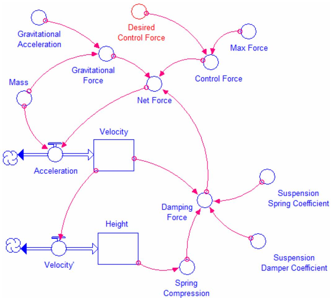
**Figure 2:** Simplified stock-flow diagram of the soft landing model
