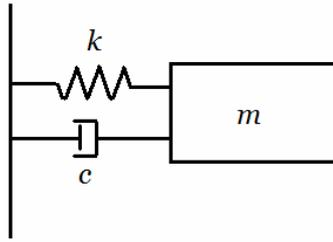
**Figure 4:** Mass spring damper schematic
