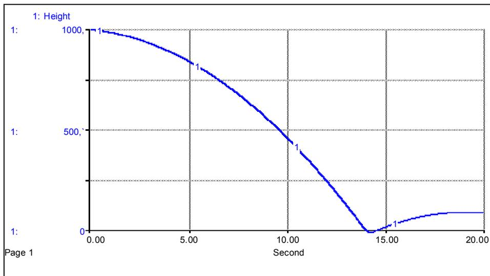
**Figure 19.** Landing behavior generated by the bang-bang heuristic in the presence of actuator delay
