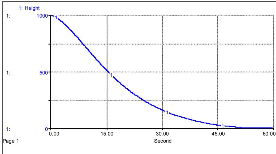
**Figure 16.** Landing behavior generated by the MSD heuristic in the presence of an error in *Height* readings
