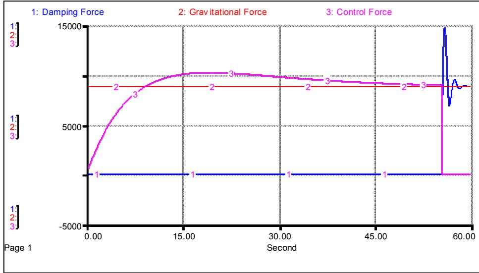
**Figure 9:** Absolute values of the forces acting on the vehicle during landing<sup>5</sup>
