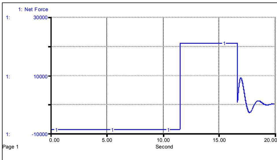
**Figure 12.** Net force acting on the vehicle during landing
