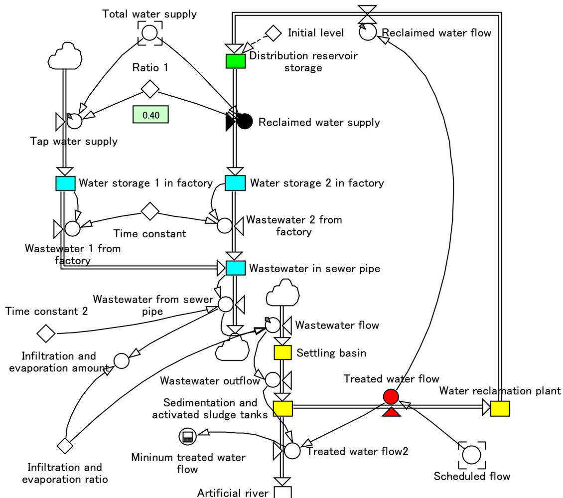
Fig. 2 System Dynamics model for analyzing water flow.
