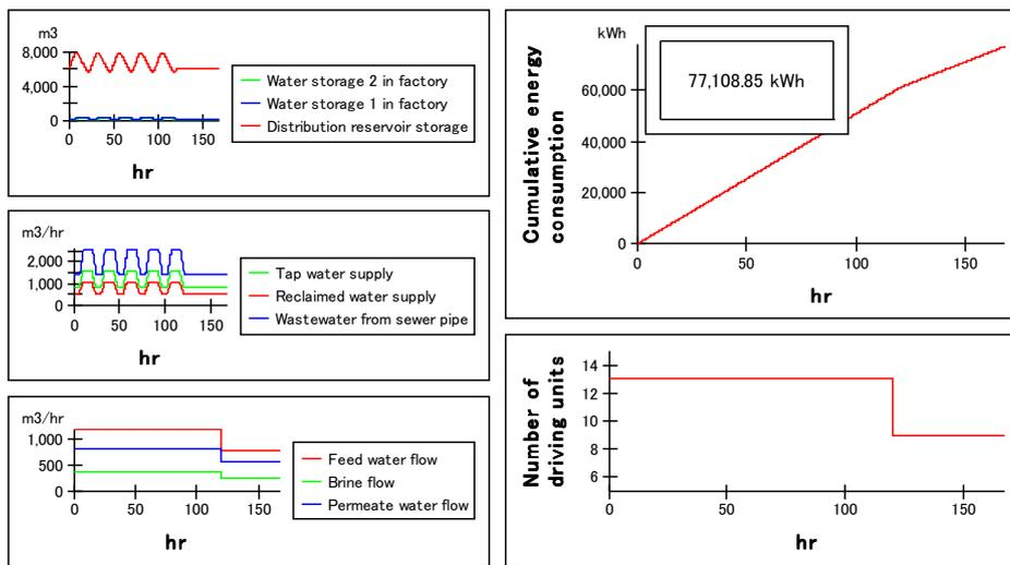
Fig. 10 Simulation example of energy consumption of RO plant.
