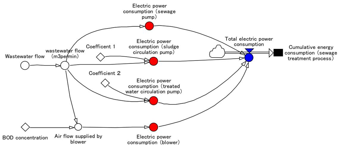
Fig. 7 System Dynamics model for analyzing energy consumption for sewage treatment process including activated sludge treatment process.
