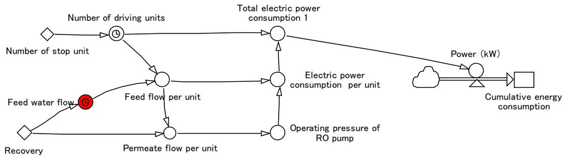
Fig. 9 System Dynamics energy model of RO plant.
