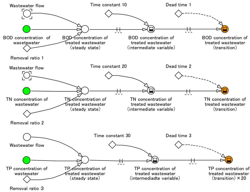
Fig. 11 System Dynamics model 1 for analyzing water quality.
