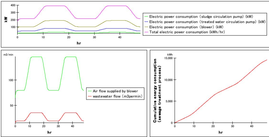
Fig. 8 Simulation example of energy consumption of sewage treatment plant.
