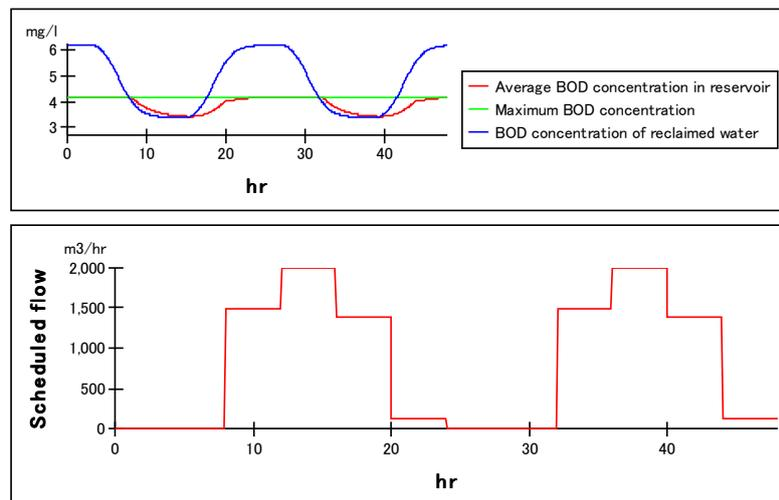
Fig. 14 Example of optimal scheduling of treated water supply.
