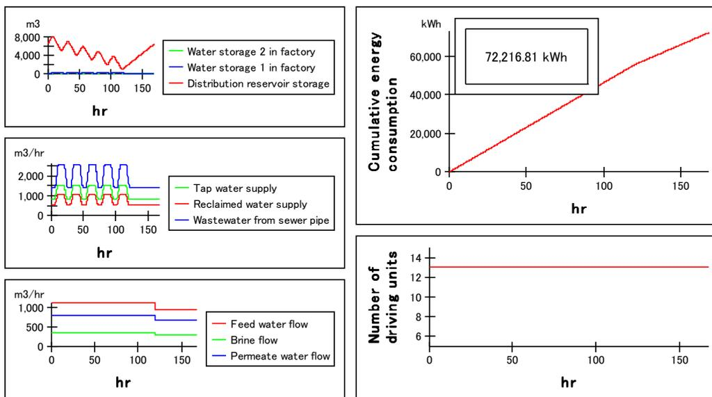
Fig. 16 Example 2 of scheduling of feed flow to RO plant.
