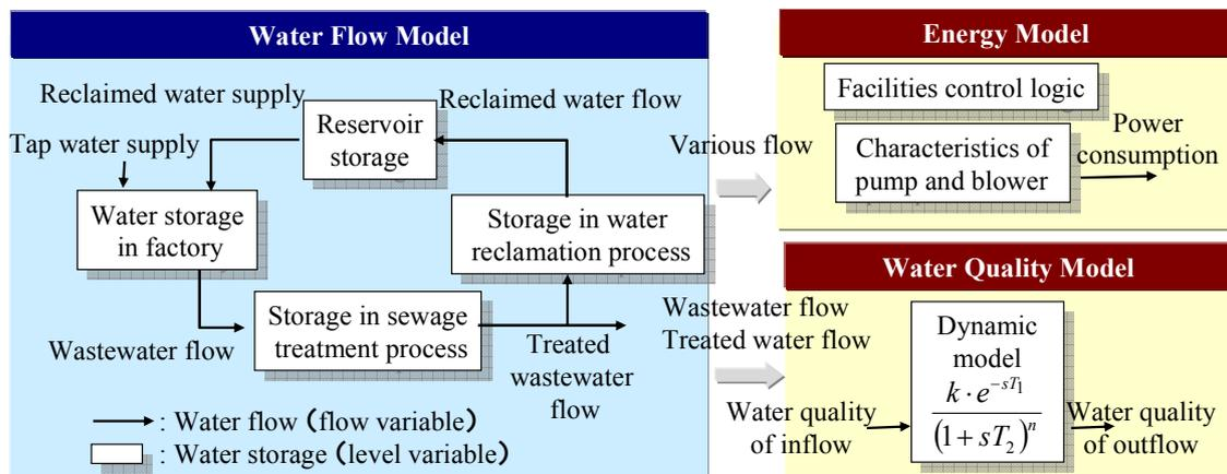
Fig. 1 Overall structure of water cycle analysis System Dynamics model.
