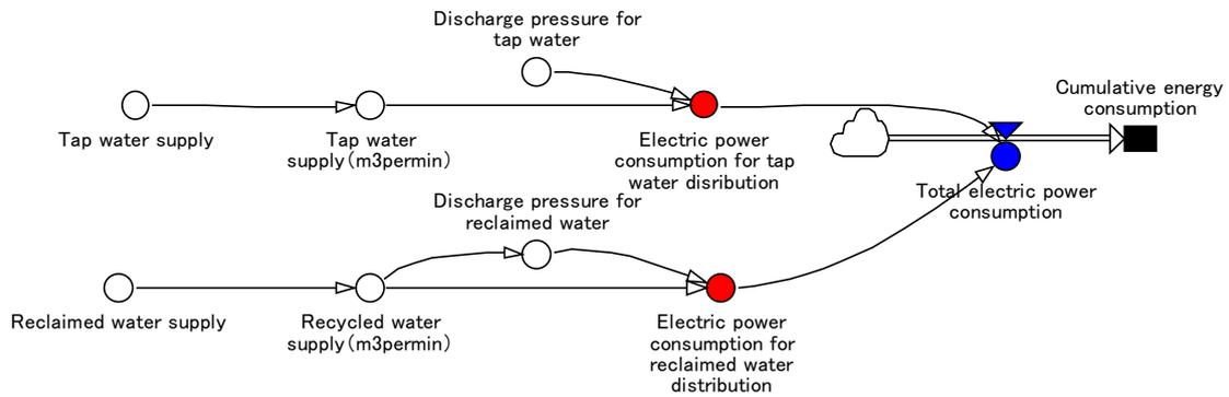
Fig. 5 System Dynamics model for analyzing energy consumption of water distribution pump.
