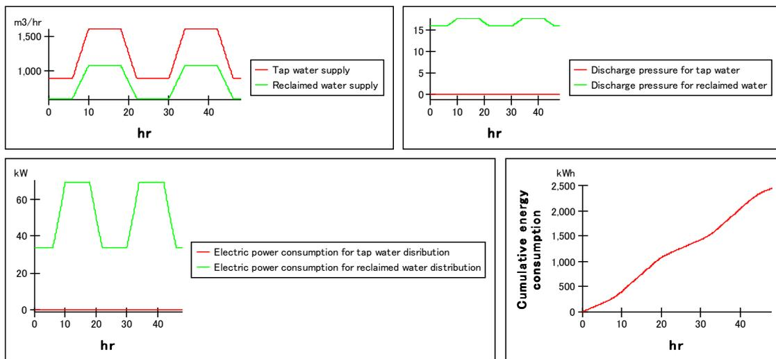
Fig. 6 Simulation example of energy consumption of water distribution pump.
