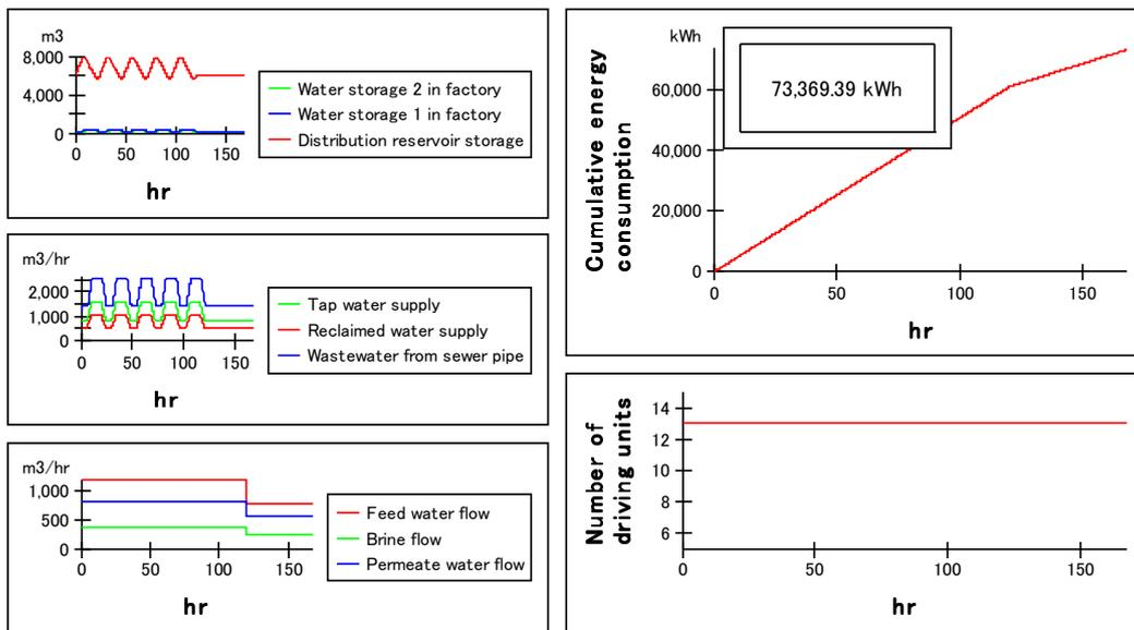
Fig. 15 Example 1 of scheduling of feed flow to RO plant.
