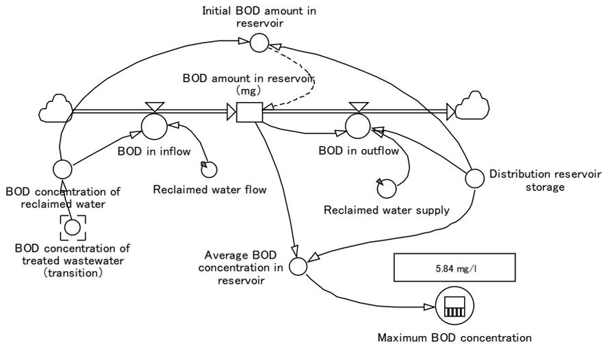
Fig. 12 System Dynamics model 2 for analyzing water quality.
