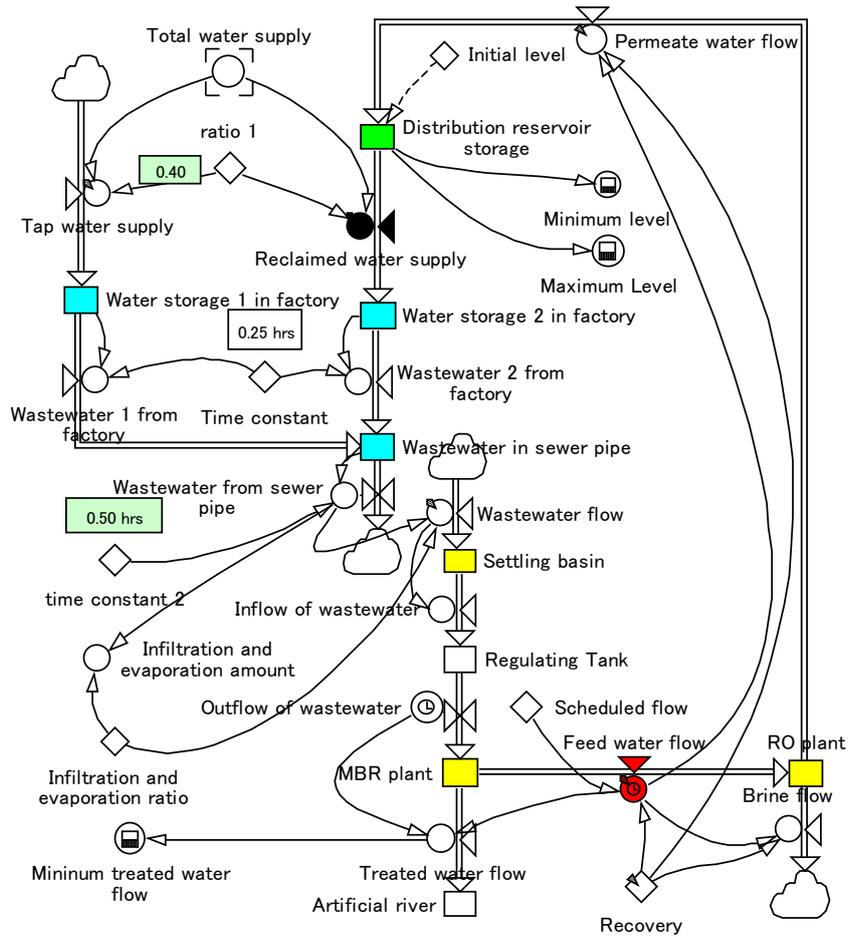
Fig. 4 System Dynamics flow model of water cycle system with MBR and RO plant.
