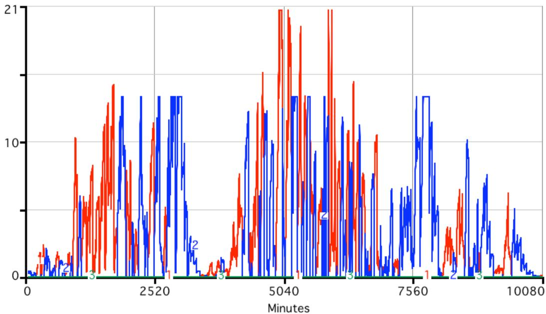
Figure B-4. Pump flows (in red) and generator flows (in blue) during a week of high water flows and hourly scheduling in a 30-minute persistence scenario. (The flows are displayed with the vertical axis scaled from 0 to 21 KCFS.)
