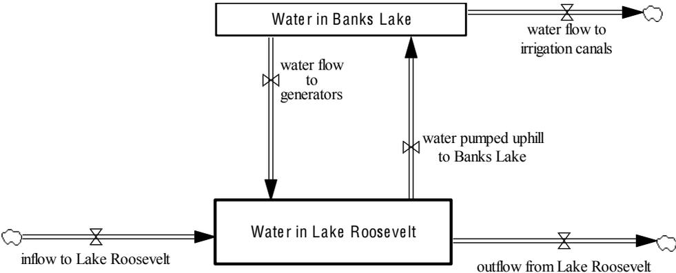
Figure B-1. Water flows and storage at the pumped storage facility.
