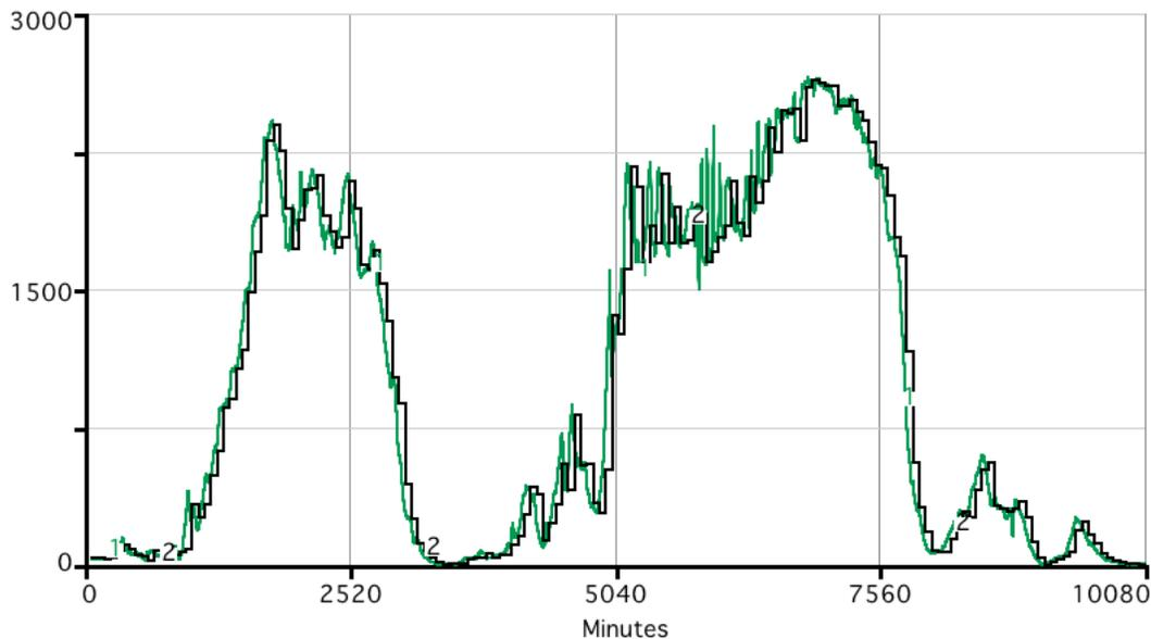
Figure B-3. Actual wind generation (in green) and scheduled wind generation (in black) during a week of high water flows and hourly scheduling in a 30-minute persistence scenario. (Results are displayed with the vertical axis scaled from 0 to 3,000 MW.)
