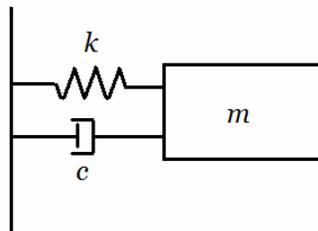
Figure 7: Mass-spring damper model
