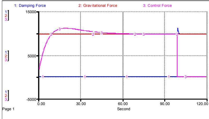
Figure 6: Absolute values of the forces acting on the vehicle during landing
