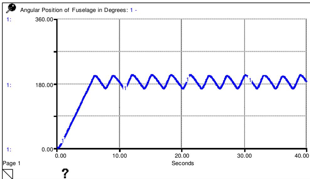
**Figure 10 :** Angular position of fuselage with Modified-VSL under delayed setting
