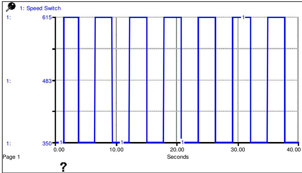
**Figure 6** : Rotational speed selections for the tail rotor with naive heuristic under delayed setting
