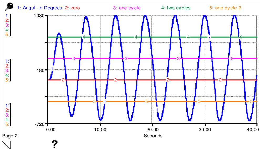
**Figure 5** : Angular position of fuselage with naive heuristic under delayed setting
