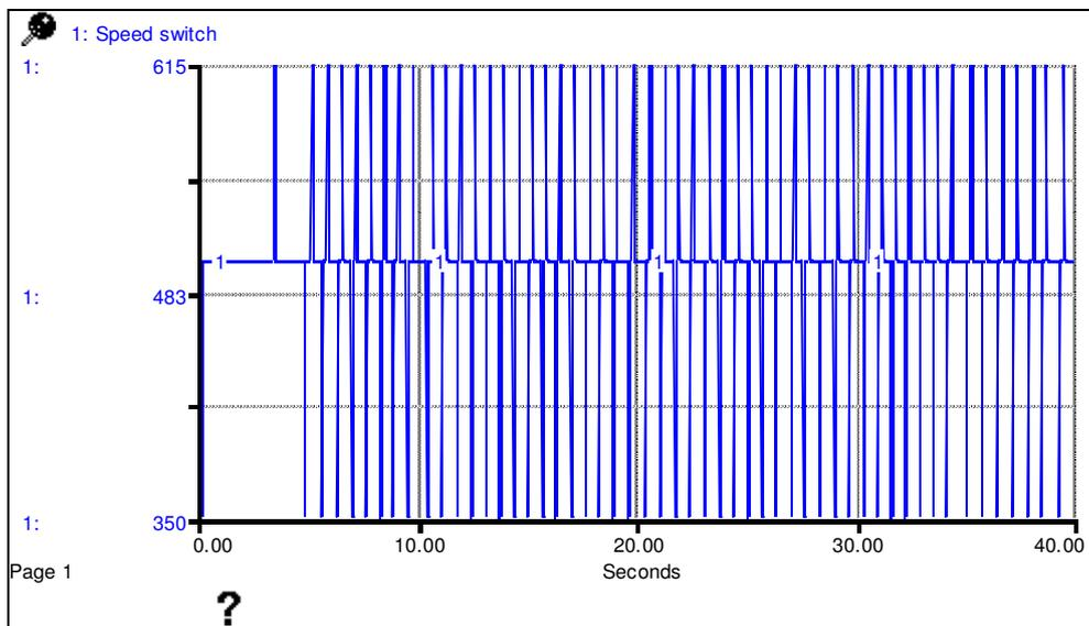
**Figure 9 :** Rotational speed selections for the tail rotor with Modified-VSL under no delay setting
