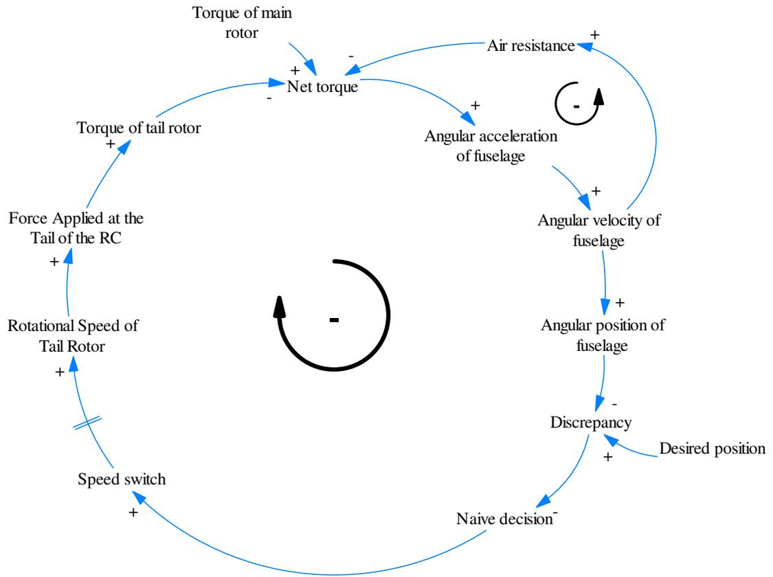
Figure 2 : Causal loop diagram for naive heuristic
