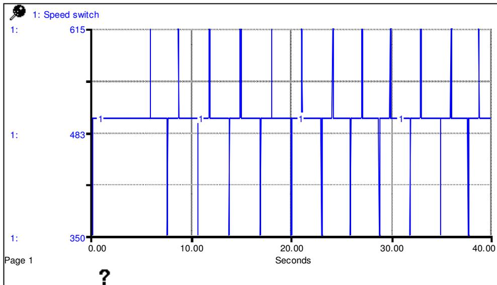
**Figure 11** : Rotational speed selections for the tail rotor with Modified-VSL under delayed setting
