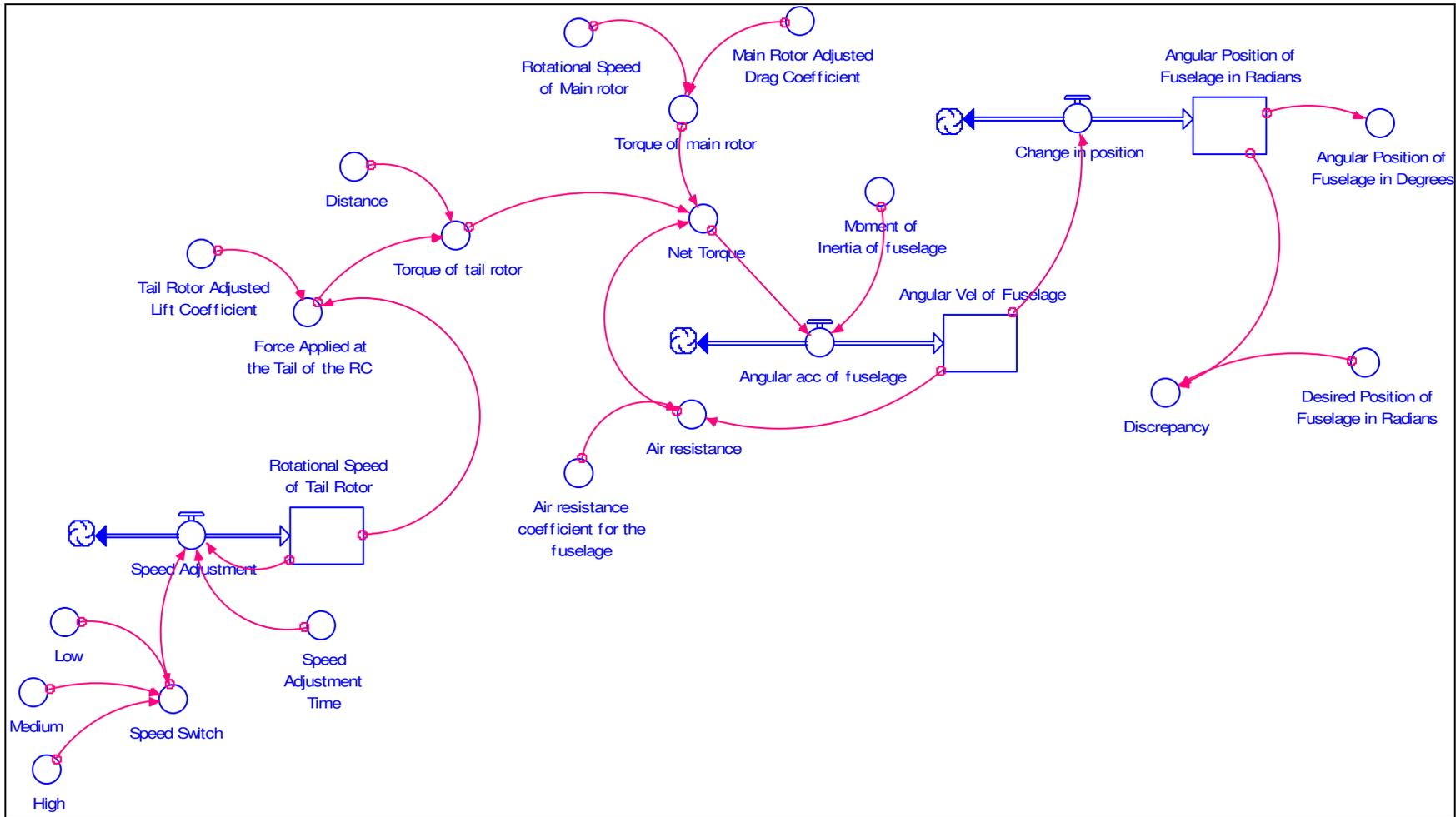
**Figure 1** : Stock-flow diagram of the model
