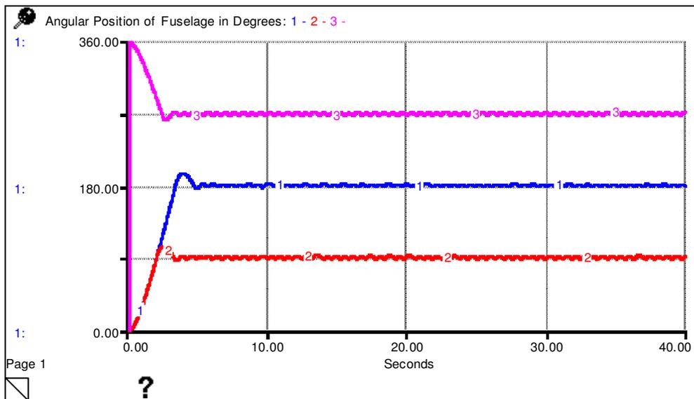
**Figure 13 :** Angular position of fuselage with Modified-VSL under no delay setting (*Discrepancy* calculations is based on a modular formulation)
