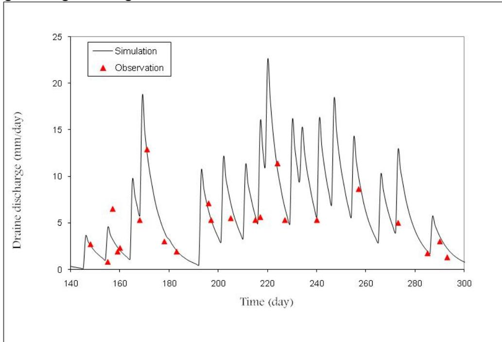
Fig. 4. The comparison between simulated and measured drain discharge
