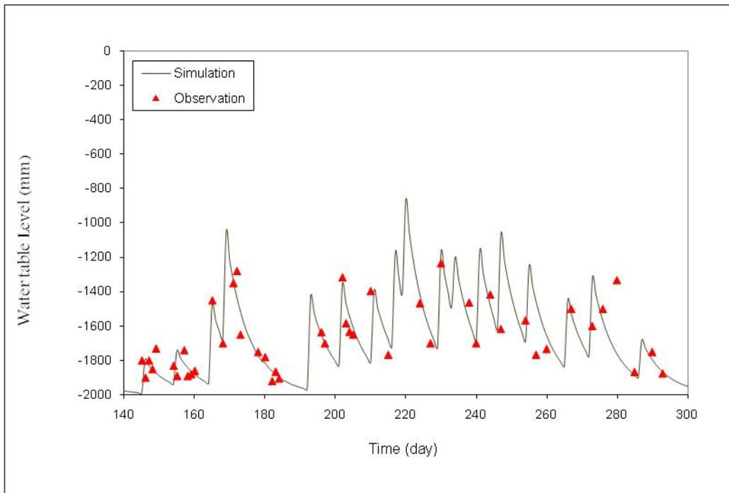
Fig. 3. The comparison between simulated and measured average water table levels
