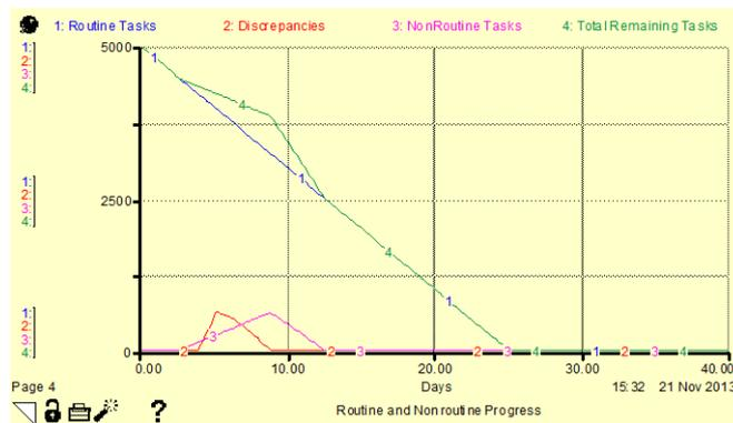
Figure 14 Routine and Non-routine tasks (50% workforce allocated to Routine)
