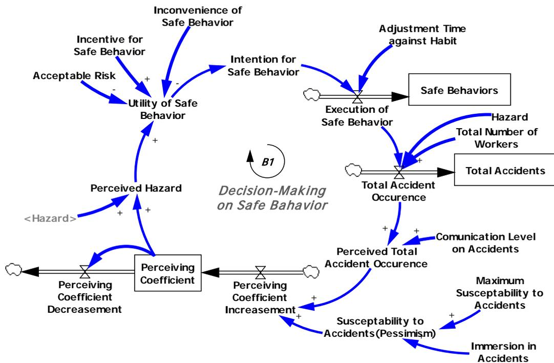
**Fig.5** Model for Worker’s Decision-Making on Safe Behavior
