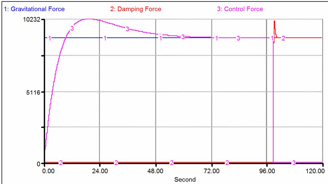
**Figure 7:** Absolute values of the forces acting on the vehicle during landing<sup>5</sup>
