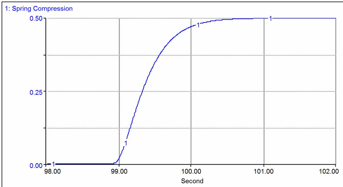
**Figure 8:** Dynamic behavior of *Spring Compression* during the final process of landing (between seconds 98-102)
