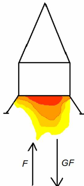
**Figure 1:** Free body diagram of the vehicle with a control force ( $F$ ) generated by the reverse force thruster and the gravitational force ( $GF$ )
