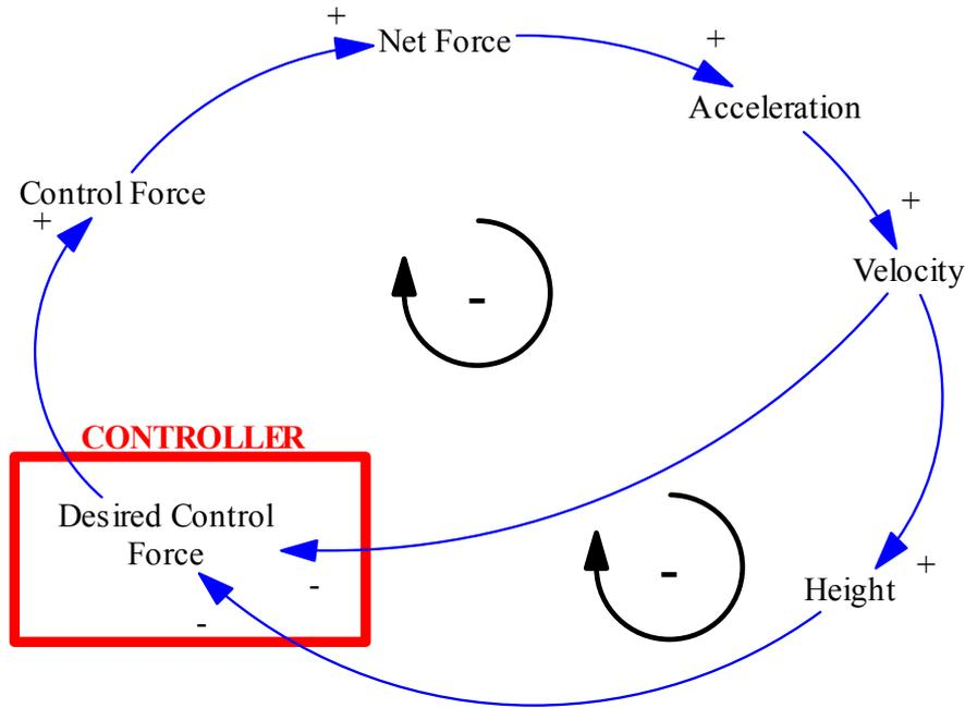
**Figure 3:** Causal-loop diagram of the control feedback loop structure
