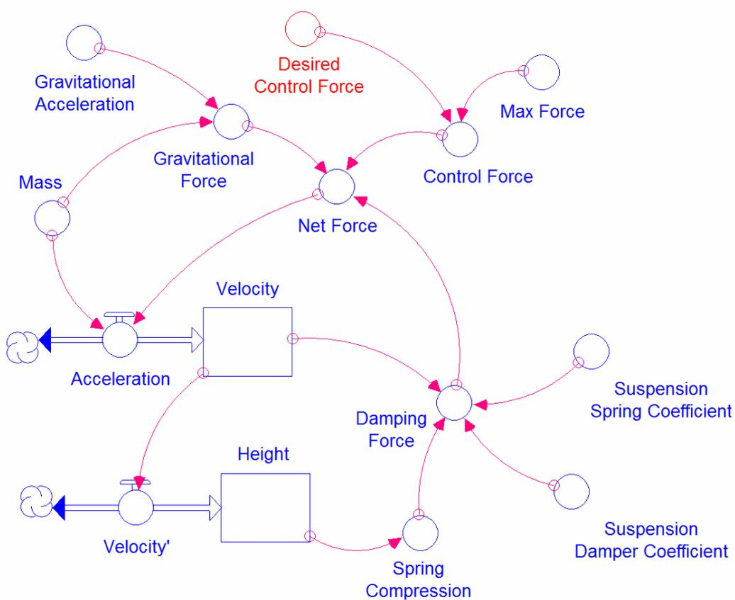
**Figure 2:** Stock-flow diagram of the model
