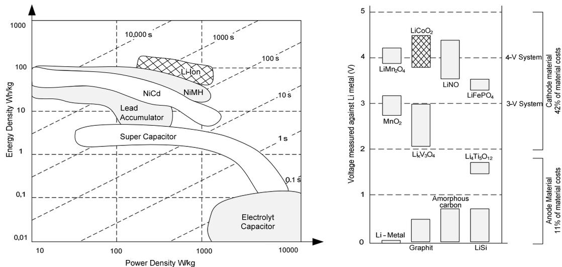
Figure 1: Energy and power densities of batteries and capacitors (KETTERER 2009)
