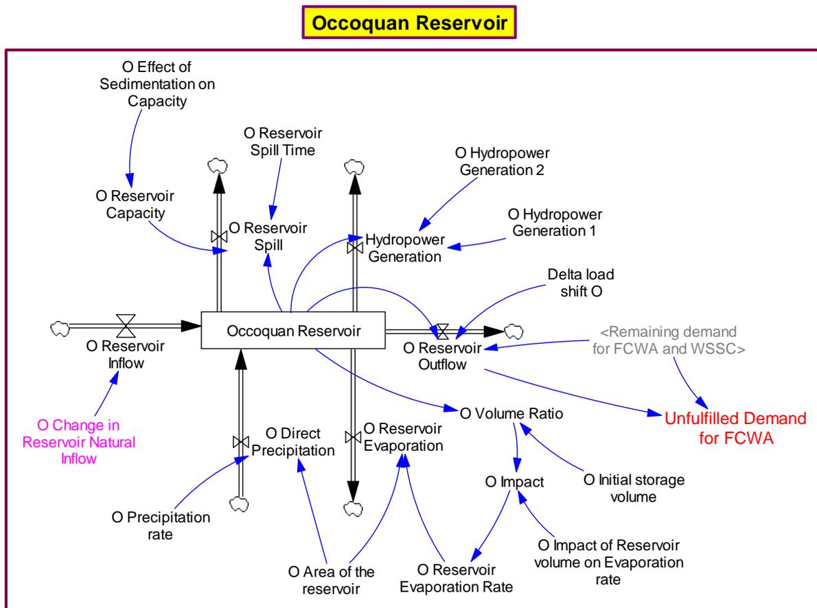
Figure 7: Supply Side Model: Occoquan Reservoir System
