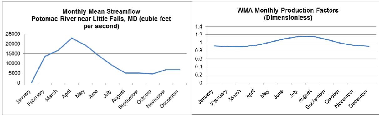
Figure 4: Monthly Mean Stream Flow for the Potomac River near Little Falls<sup>3</sup>, WMA Monthly Production Factors
