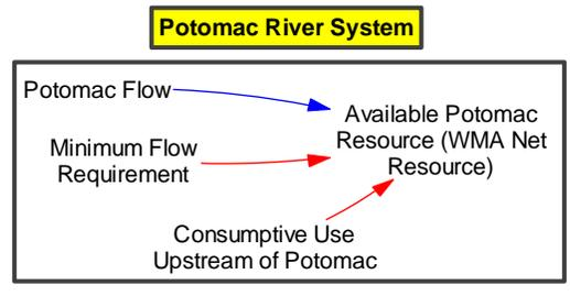
**Figure 6: Supply Side Model: Potomac River System**
