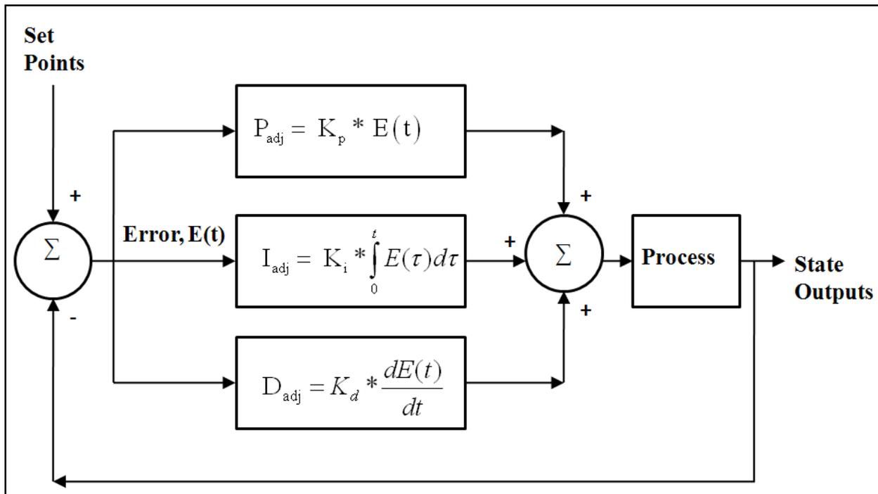
**Figure 1:** Proportional-Integral-Derivative (PID) feedback structure
