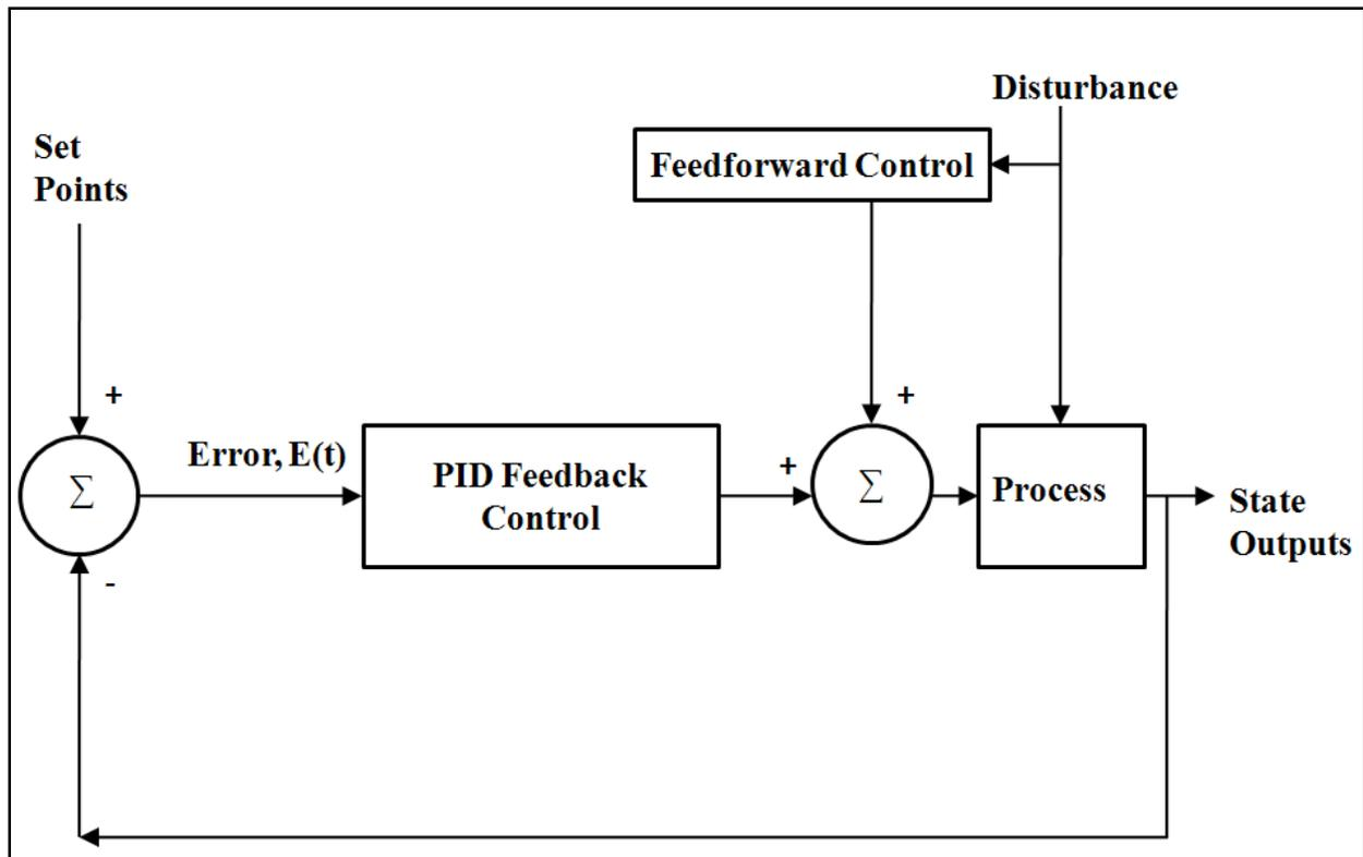
**Figure 2:** Combined feedback-feedforward control structure
